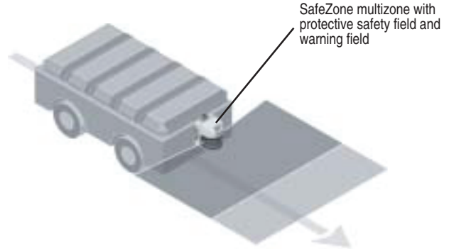
Figure 56: Vehicle monitoring with SafeZone safety laser scanner
